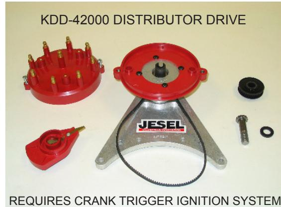
JESEL ALSO OFFERS A DISTRIBUTOR DRIVE KIT FOR THE BIG-BLOCK CHEVY. THE DISTRIBUTOR DRIVE KIT ELIMINATES INACCURATE IGNITION TIMING SETTINGS DUE TO CAMSHAFT TORSIONAL TWISTING ON HIGH RPM ENGINES WITH EXCESSIVE SPRING PRESSURES. IT ALSO PROVIDES A MUCH COOLER LOCATION FOR THE DISTRIBUTOR. INTAKE MANIFOLD CHANGES WILL BE MUCH EASIER AS WELL THANKS TO THE DISTRIBUTOR NOT HAVING TO BE ROUTED THROUGH THE REAR PORTION OF THE INTAKE MANIFOLD. THIS KIT IS A DIRECT BOLT ON.
